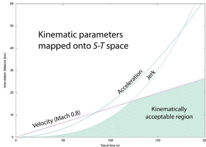
**Figure 2.** Velocity, acceleration, and jerk parameterized in terms of inter-station separation  $S$  and travel time  $T$ . In the region below each curve the kinematic constraints (vi) are met. The hatched area is the region where all constraints are simultaneously met.
